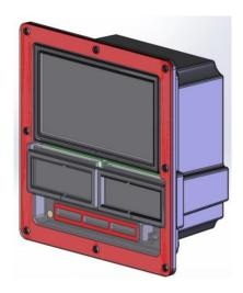
Although the CI515 Preset Board is optionally housed in the TP Slave Display enclosure, there is no direct connection with other boards in the enclosure other than the BUS connector. In the same manner as the CI507 Temp-Press Main Board, the CI515 Preset Board is provided with BUS-IN and BUS-OUT connections J100 and J101 respectively. The CI515 Preset Board takes input from the keypad(s) and provides information on the RS485 lines on the BUS.
