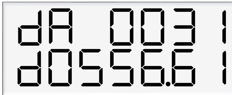
The electronic totes can also be viewed by pressing the # key five times on the main display, as long as the unit is not in a transaction. Each tote will be shown for ten seconds before the next tote is displayed.
