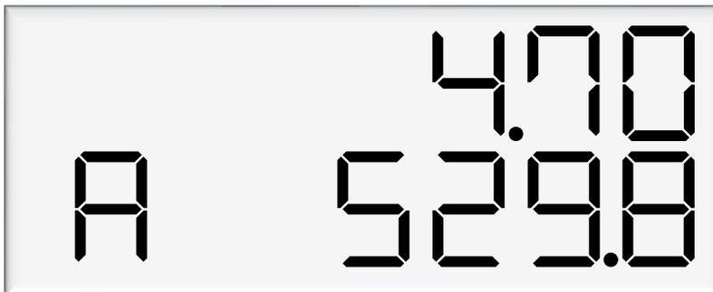
The top row will show uncompensated, unsuppressed quantity dispensed in litres, while the bottom row will show the density reading at 15°C. The unit price display will show the temperature reading at the end of the sale. The left most character of the density reading indicates the nozzle side.
