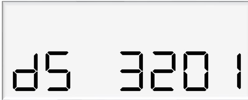
Slave display numbers can be set with switches 2 and 3 on the slave display board. Use the following table to configure slave display numbering.
