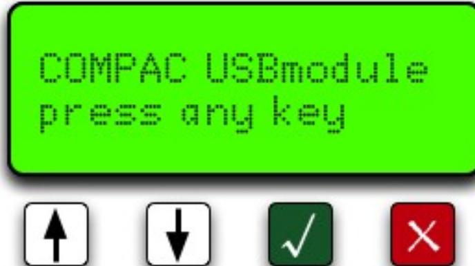
Plug your USB stick into the USB slot and push any of the keys. It will then display "Searching USB...".
