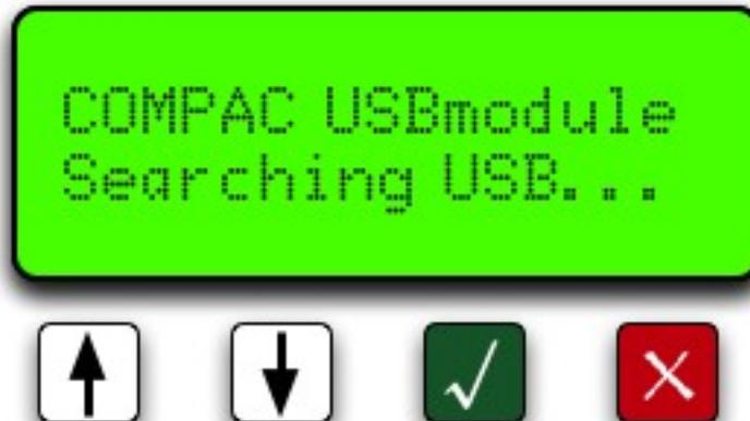
If the USB stick does not contain the Compac USB security code the display will read "Non Secure USB". You will have to load the "USB Key" file onto the key before it will work.
