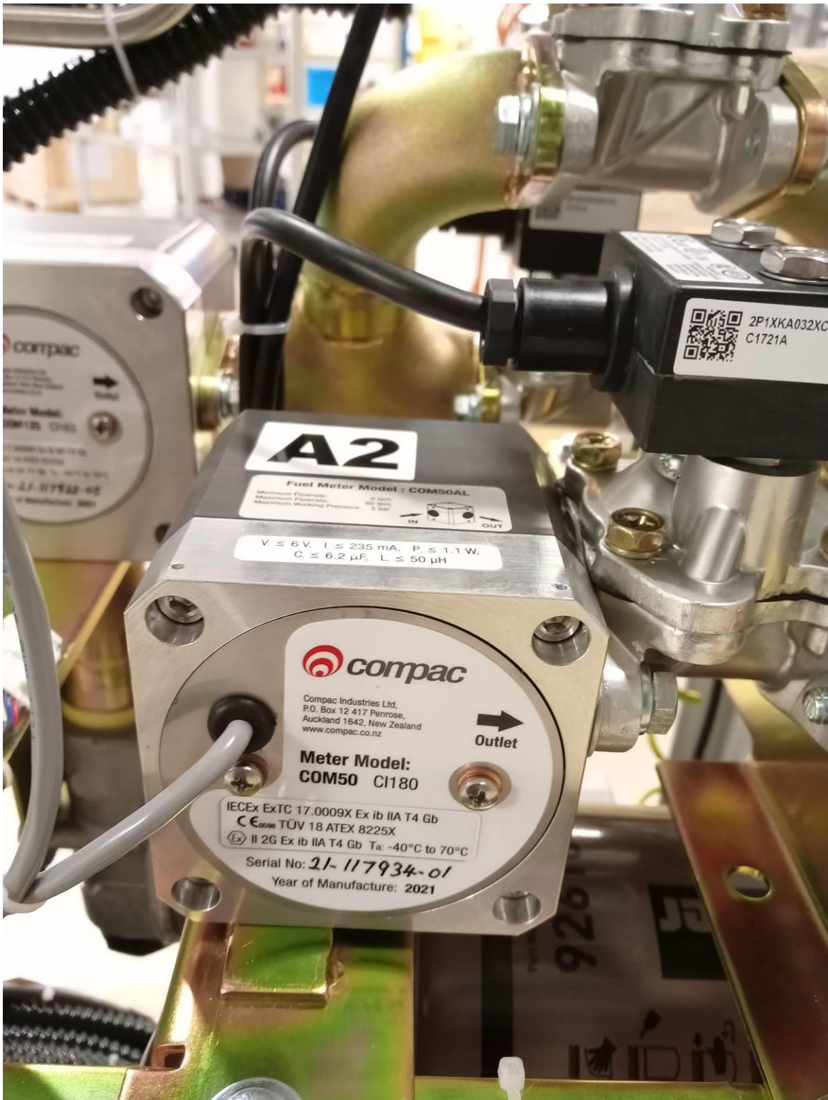
Compac COM-50 flowmeter with anodised aluminium housing (Variant 18)
