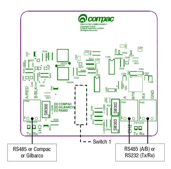
Switches 300, 302, and 303 are for RS485/RS232 Terminator application. Use the following table to configure these switches. Switch 300 is for channel 1, and switches 302 and 303 are for channel 2.
