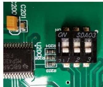
**CAUTION :** Make sure the device is powered off before attempting to change the dip switches
