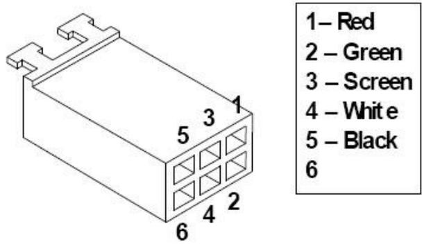
Figure 3: Connector from CI 214 J8 to C4000
