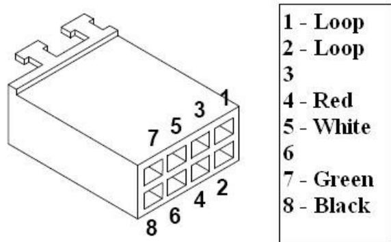
Figure 4: Connector to Temperature Compensation PCB (Con 5)
