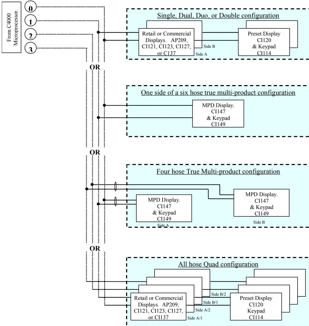
Figure 18. Display Connections for Various Dispenser Models.
