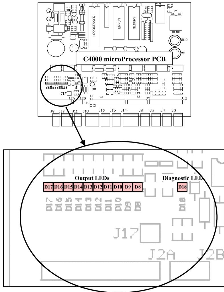
Figure 6. Location of Output & Diagnostic LEDs
