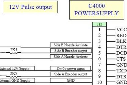
**NOTE** If a Triscan unit is not connected to the Pump or Dispenser, "Standalone operation" can be achieved by "shorting" Triscan Switch A (terminal "CTS"), & Triscan Switch B (terminal "DTR") to terminal "GND" & linking terminal "VCC" to terminal "TXDP". This must not be done if a Triscan unit is connected.
