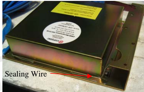
Fig. 2 Sealing of C4000 Processor Cover
