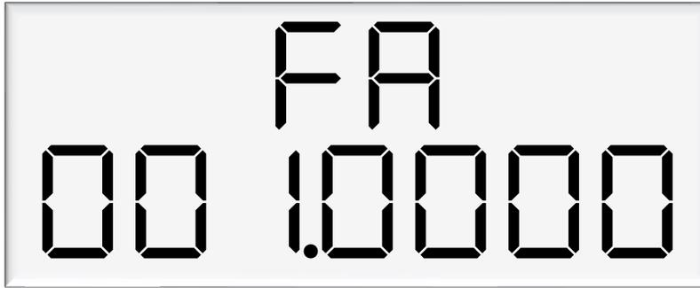
The K-Factor is used to calibrate the dispensers KG100 meter with a master meter or meter prover (Scales). See meter calibration for more details on calibrating the dispenser
