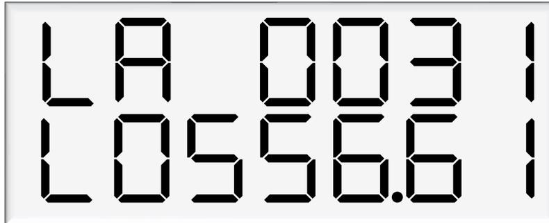
The bottom row is a continuation of the top row – for example, the above display should be read as 003 10556.6 |. The side (A or B) will be shown in the unit price display. Dollars totals are also recorded, which can be viewed by continually pressing the parameter switch.
