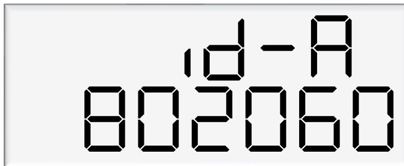
To set the meter id Each press of the K-Factor switch passes you over a digit, making the digit blink. Holding the switch down for more than a second changes whichever digit is currently displayed. If you want to pass over a setting without changing any digits, keep pressing and releasing the switch.
