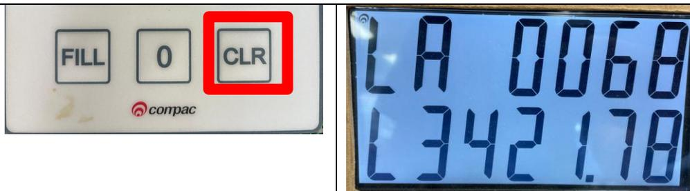
Enter the Passcode for the dispenser. The preset keypad will beep every time a button is preset to indicate a button was pressed.
